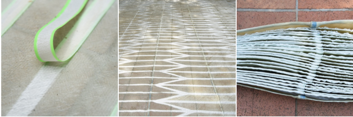
Figure 2: The fabrication process allows the structure to flat-pack to less than a 12" width.
